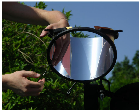
Fig. 70: Secondary reflector fixation
