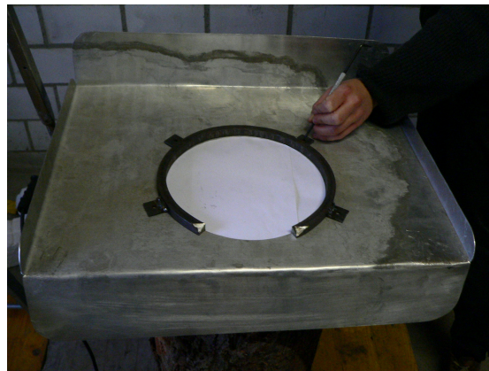
Fig. 64: Marking holes for C11
