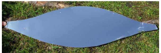
Fig. 69: Shape Secondary Reflector, according to latitude.
