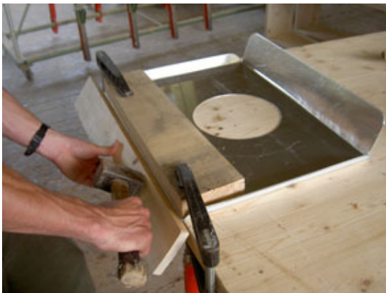
Fig. 63: Making of aluminium cooking surface
