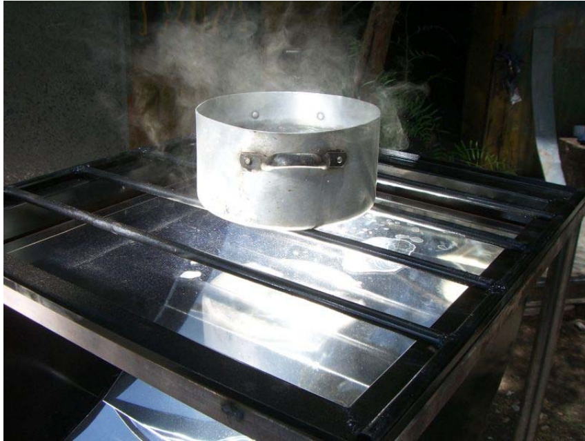
Fig.6: Ceramic glass as protection for the secondary reflector (better use black pots ;-))
