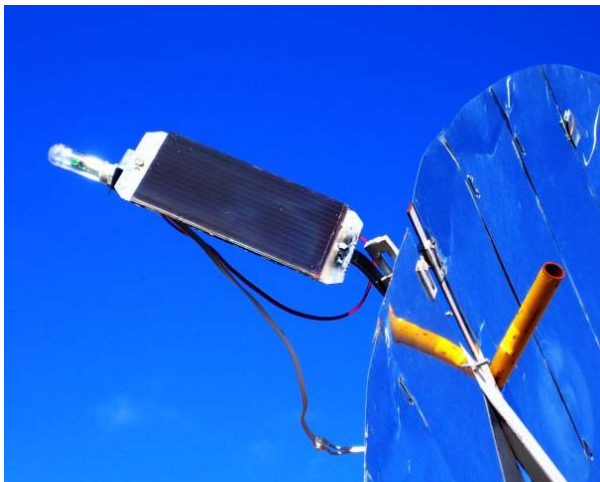
Fig. 8: Solar panel with electronics
